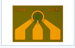
Cosemi's LPD3010 is a mesa-structured, InGaAs/InP-based PIN photodiode offering high responsivity, low dark current and low capacitance for high bandwidth, high performance optical receiver designs.
